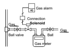
Scheme for installation of the solenoid valve
